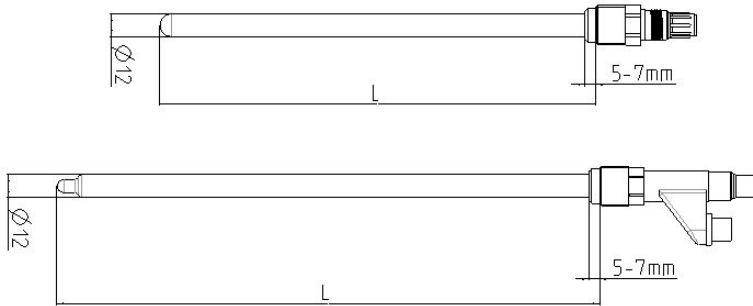
Fig. 4: Sensor filled with gel (on top) Sensor filled with liquid (below)
