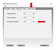
The output value for the detection of a transmitter error is adjustable between 3.5...22.5 mA.
